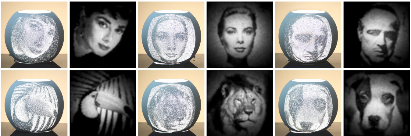
Fig. 16. Additional results on spherical lampshades. Left: our 3D-printed lampshade, with light projecting through the surface. Right: the photo of projected image. The lamps are 22cm in diameter.
