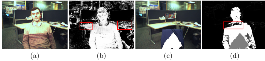
Fig. 1. The error caused by ambiguous colors. (a) input image; (b) probability map produced by the global color model (a pair of GMMs learned according to the ground truth of (a)), the pixels with greater intensity are more likely to be foreground; (c) the background image. Note that the background image is incomplete (in the large white region), and the reason is explained in section 4; (d) the result of background subtraction. From (b)(d) one can find a lot of misclassified pixels due to ambiguous colors (in the red rectangles).
