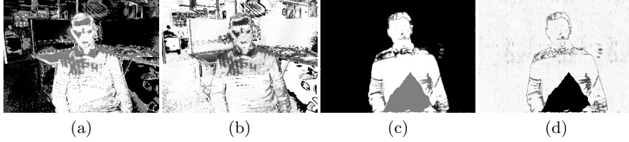
Fig. 2. Probability and confidence map. The input image is the same as in Fig.1. (a) detected misclassified pixels (the gray pixels); (b) confidence map of the global color model (visualized in Fig.1(b)), greater intensity implies higher confidence; (c) probability map produced with our per-pixel color model; (d) confidence map of (c).
