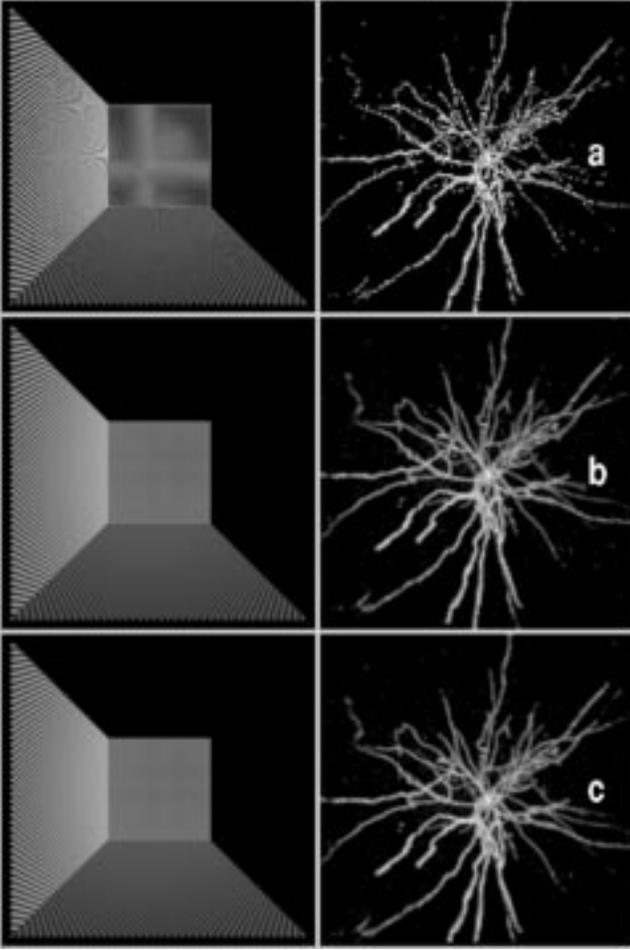
Figure 7: The left column is a  $256^3$  test volumes with  $3^3$  sub-cubes with the eye at  $(128, 128, -128)$  and 90 deg field-of-view. The right column is the LGN dataset. Row (a) Undersampling, (b) ER-Perspective, (c) Oversampling.
