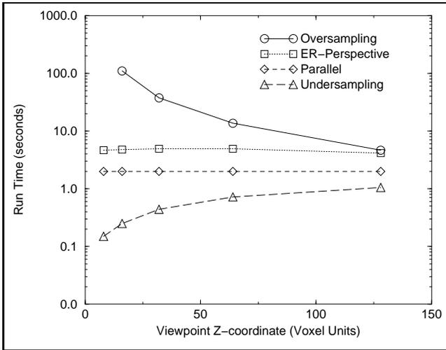
Figure 9: *Runtimes for each of the algorithms for a  $125^3$  LGN neuron volume as the distance from the viewpoint to the front of the volume changes. The algorithms ran with a high-quality full Phong equation look-up-table shading of every sample point.*
