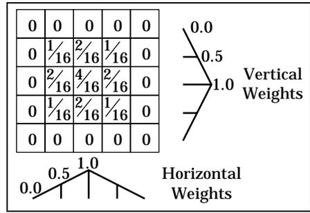
Figure 3: 2D filter of size  $\pm 2$  samples. The filter is a linear ramp in each dimension. To generate a 2D filter, the weights are multiplied and then normalized.
