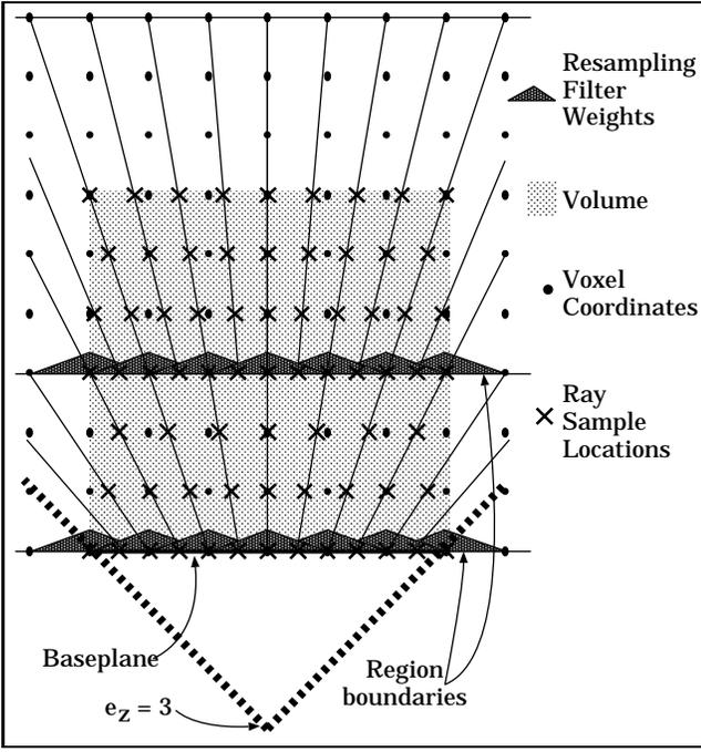
Figure 4: A  $7^3$  volume, where the viewpoint is 3 voxel units in front of the volume. The rear of the volume does not coincide with a region boundary, but the rays are still positioned on the voxel coordinates at the rear of the region boundary. In this example the view frustum is set up so that the final image coincides with the baseplane
