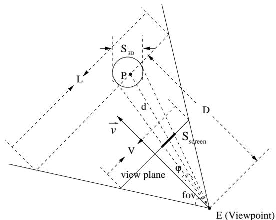
Figure 4: Estimation of point's screen projection size.
