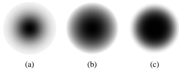
Figure 3: *Alpha textures: (a) Gaussian  $e^{-\frac{r^2}{2\delta^2}}$  ( $\delta = 0.4$ ), (b)  $1 - r^2$ , and (c)  $(\cos\pi r + 1)/2$ , where  $r$  is the radius and alpha is 0 if  $r > 1$ .*
