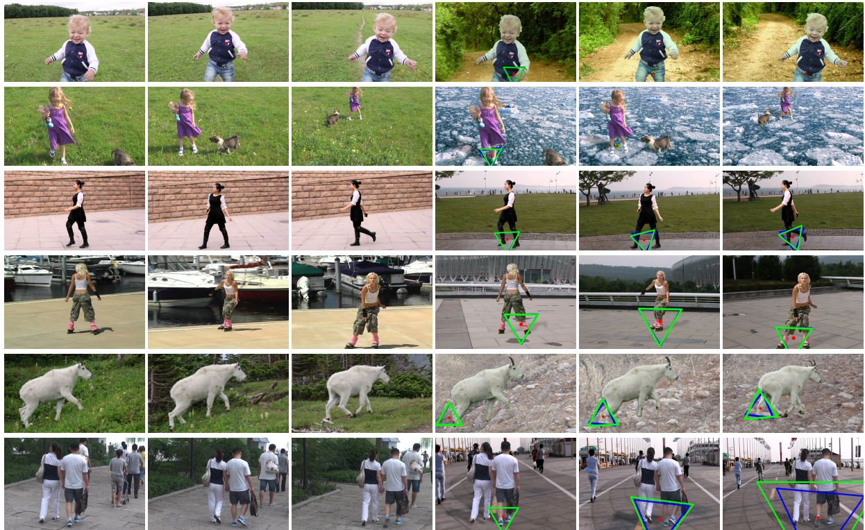
Figure 11: Results, from top to bottom: BOY, GIRL, WALK, SKATER, GOAT, COUPLE. Left: source frames (frame 10, 100, and 200). Right: The corresponding frames with new background. The green and blue triangles are the transforming triangles of the source and the result, respectively. The source videos of BOY, GIRL, SKATER, GOAT were obtained from pond5.
