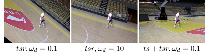
Figure 10: Effect of using the hybrid warp model. The shown image is frame 260 of BASKETBALL. Using only tsr warping results in excessive rotation, even when \omega^d is set to be very large.
