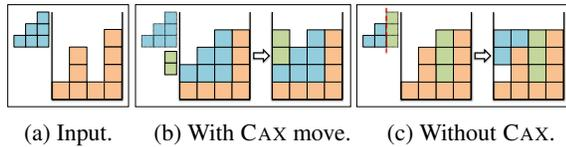
**Figure 17:** Allowing the pile to be partially flattened by making a cut, a CAX move, leads to a better DAP solution. Compare results in the middle and right where the same number of parts are obtained. With a CAX, we obtain a packing without gap.
