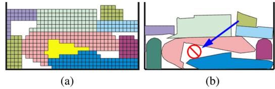
**Figure 11:** Sub-optimality of the global and local DAP optimizations. (a) With voxels employed by the global DAP step providing rather loose bounds of the actual shape pieces, the dark green voxelized piece on top could not fit in the yellow gap. The actual piece can (b). However, local refinement cannot move the piece either as only local moves (without interpenetration) are allowed.
