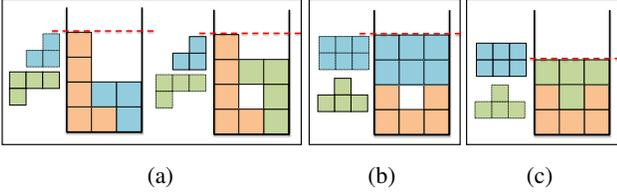
**Figure 4:** A few options to define the priority score. (a) Maximum height is oblivious to moves which do not increase the maximum height of the pile; two such moves are shown, with the left one being more desirable for packing. (b) Maximizing total height gains as the priority prefers packing larger pieces which may leave vertical gaps. (c) Combining total height gains with a penalty on vertical gaps, a compact packing with smaller pieces can win.
