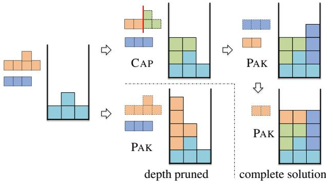
**Figure 6:** An illustration of DAP search on a minimal example for powder-based printing; arrows show the search paths. The illustration starts at a partial solution (a node in the search tree) with two pieces (left) to process. By a CAP move and two following PAK moves, the top path runs into a complete solution, while the bottom path is depth pruned, in reference to the complete solution found.
