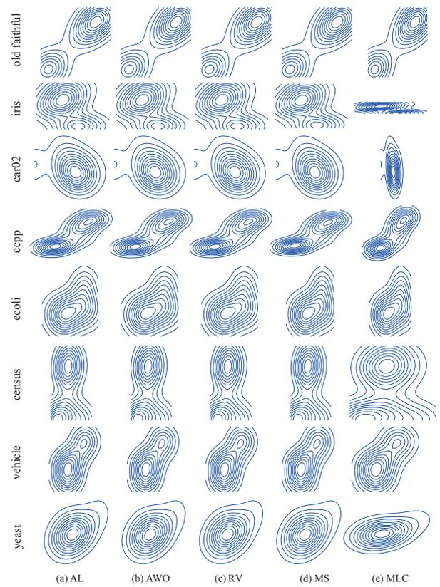
Figure 6: Selected 2D contours from Figure 4 generated by different aspect ratio selection methods. As in the case of 1D curves, AWO, RV and AL are almost the same. MS is similar to AL, but it selects slightly taller aspect ratio for *ecoli*. MLC produces smaller aspect ratios in some cases (*iris* and *census*) but selects larger ones for the other data.
