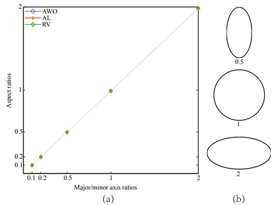
Figure 7: Comparison of AL, AWO and RV with ellipses generated by varying ratios of major to minor axis. (a) shows the relationship between the ratios of major to minor axis and the selected aspect ratios; (b) three ellipses with different ratios. The aspect ratios of all methods are almost the same, ellipses are banked to circles.
