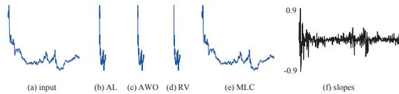
Figure 10: Banking a curve (a) where most of slope values (see (f)) are very small. AL (b), AWO (c), and RV (d) produce overly tall aspect ratios, while MLC (e) preserves the original shape.
