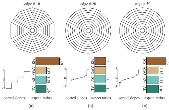
Figure 8: Comparison of the aspect ratios generated by MS, AWO, RV and AL on 2D circular contours with different discretization. MS behaves the same as AL when the number of edge is 20, while its resulted aspect ratios are taller when the number of edges are 10 and 30. In contrast, AL, AWO and RV always are very similar.
