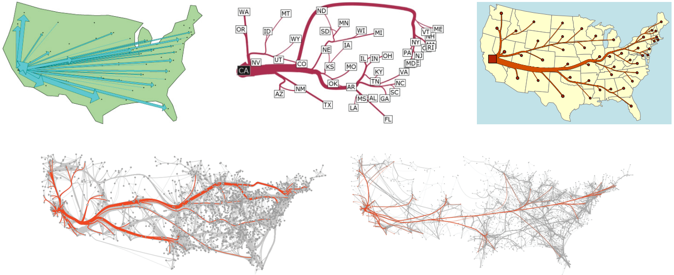
Fig. 2. Maps illustrating migration from California 1995–2000. Top: flow maps, Tobler [1, 22] (arrows of varying width), Phan et al. [16] (edge-bundling with crossings), and our output. Bottom: subgraphs of the bundled complete migration graph, Cui et al. [5] and Holten & van Wijk [11].
