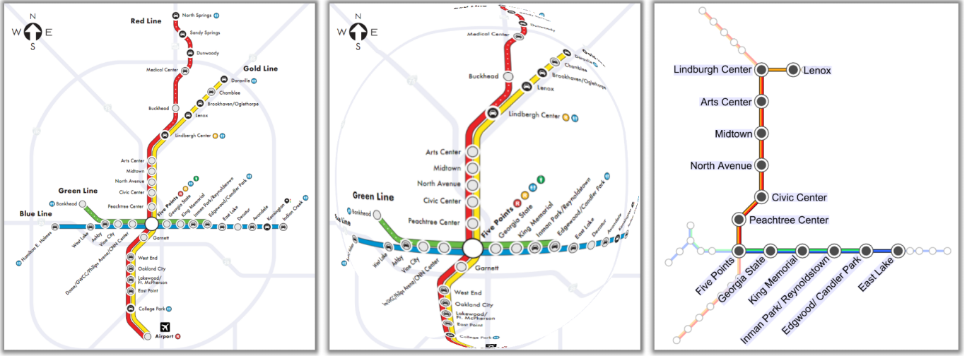
Fig. 1. (left) The official metro map of Atlanta city [18]. (middle and right) The focus+context metro maps obtained using the fisheye [22] and our method, respectively. The official map would become too small if it is displayed on a small area. In highlighting the route of a passenger, the fisheye method [22] distorts the map while our technique introduces no visual artifacts.
