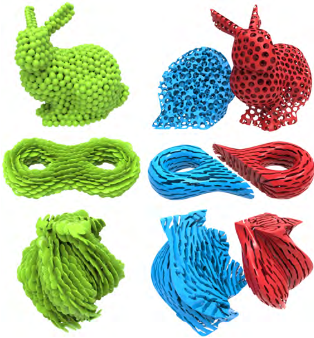
Figure 13: Results produced using different tensor field specified by users. Left: pores; Right: porous structures. Bunny: n = 1650, \rho = 65\% ; Double-torus: n = 1000, \rho = 50\% ; Vase: n = 1650, \rho = 48\% .
