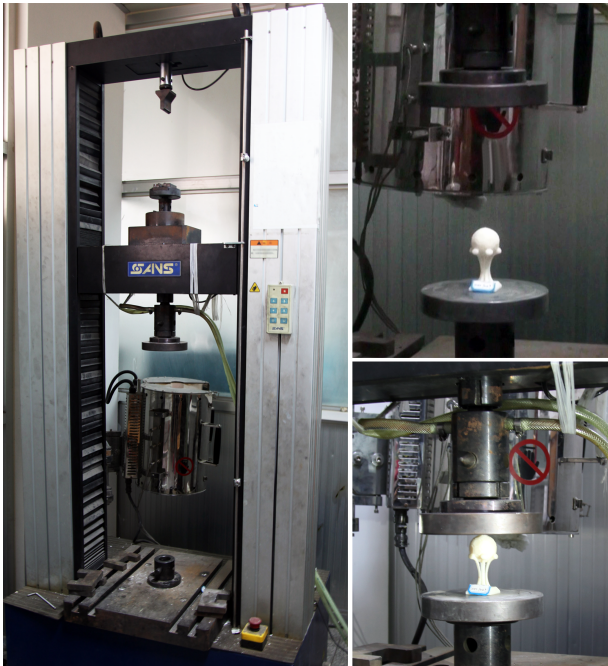
Figure 11: Compression tests using a universal testing machine.
