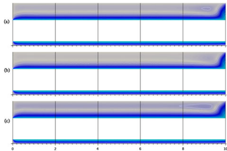
Figure 12. r_{Re} = 0.0 velocity profiles of (a) Newtonian fluid, (b) pseudoplastic fluid, and (c) dilatant fluid.
